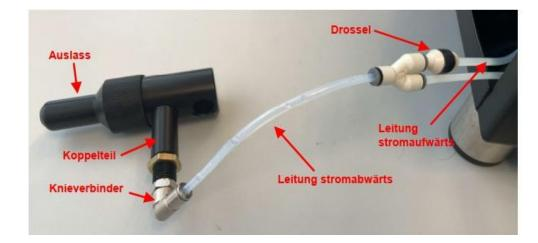
Taking into account the pipe area in the knee connector, this results in a section length with an extended diameter downstream of the throttle device of around 10 cm, as demonstrated in the following figure (note: reference symbols and length determination have been inserted by the applicant):
