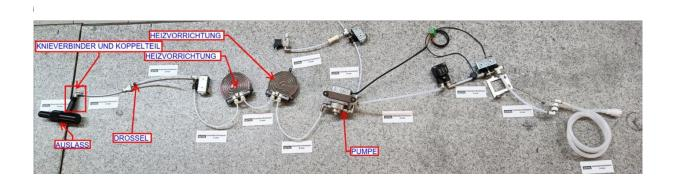
The following illustration shows that the line downstream of the choke is connected to the coupling part via a knee connector (note: reference symbols have been inserted by the applicant):
