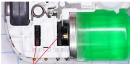
Drive wheel having two interconnected ratchet wheels
