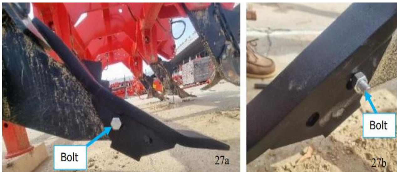
Figure 27a, 27b. Different lateral views of an alternative embodiment wherein the Bellota tool is fixed by a bolt.
