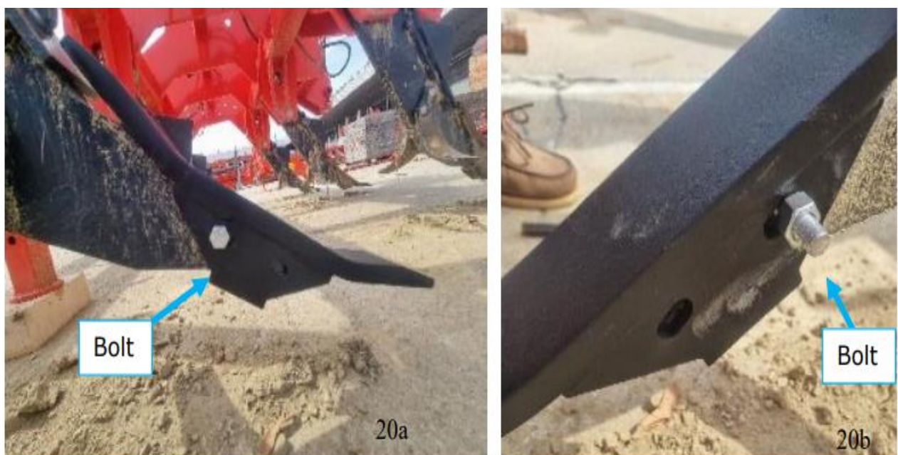
Figure 20a, 20b. Different lateral views of an alternative embodiment wherein the Bellota tool is fixed by a bolt.
