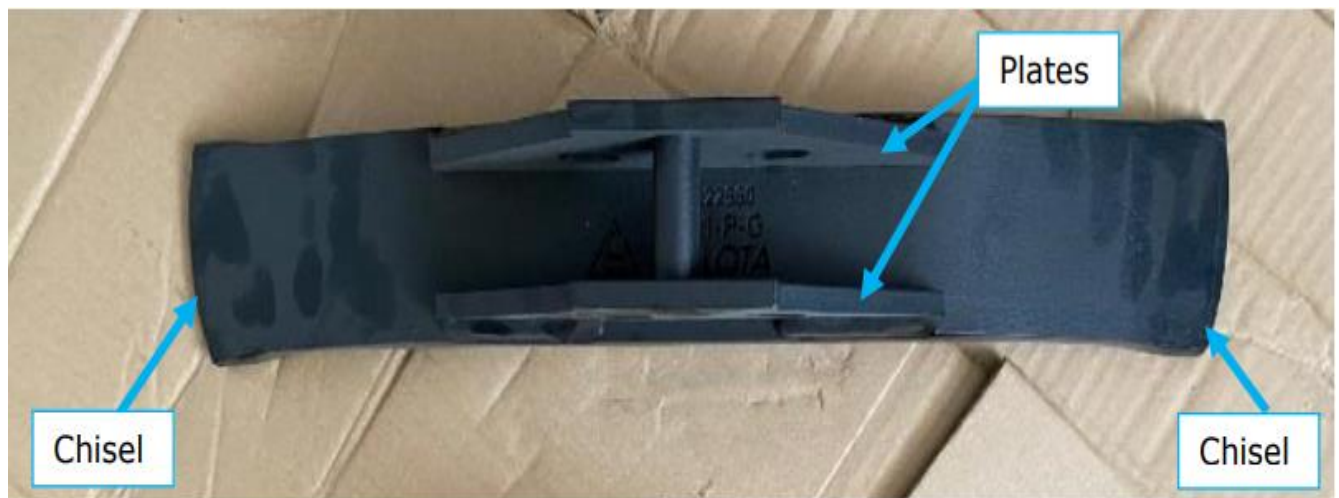
Figure 23. Top view of the Bellota tool
