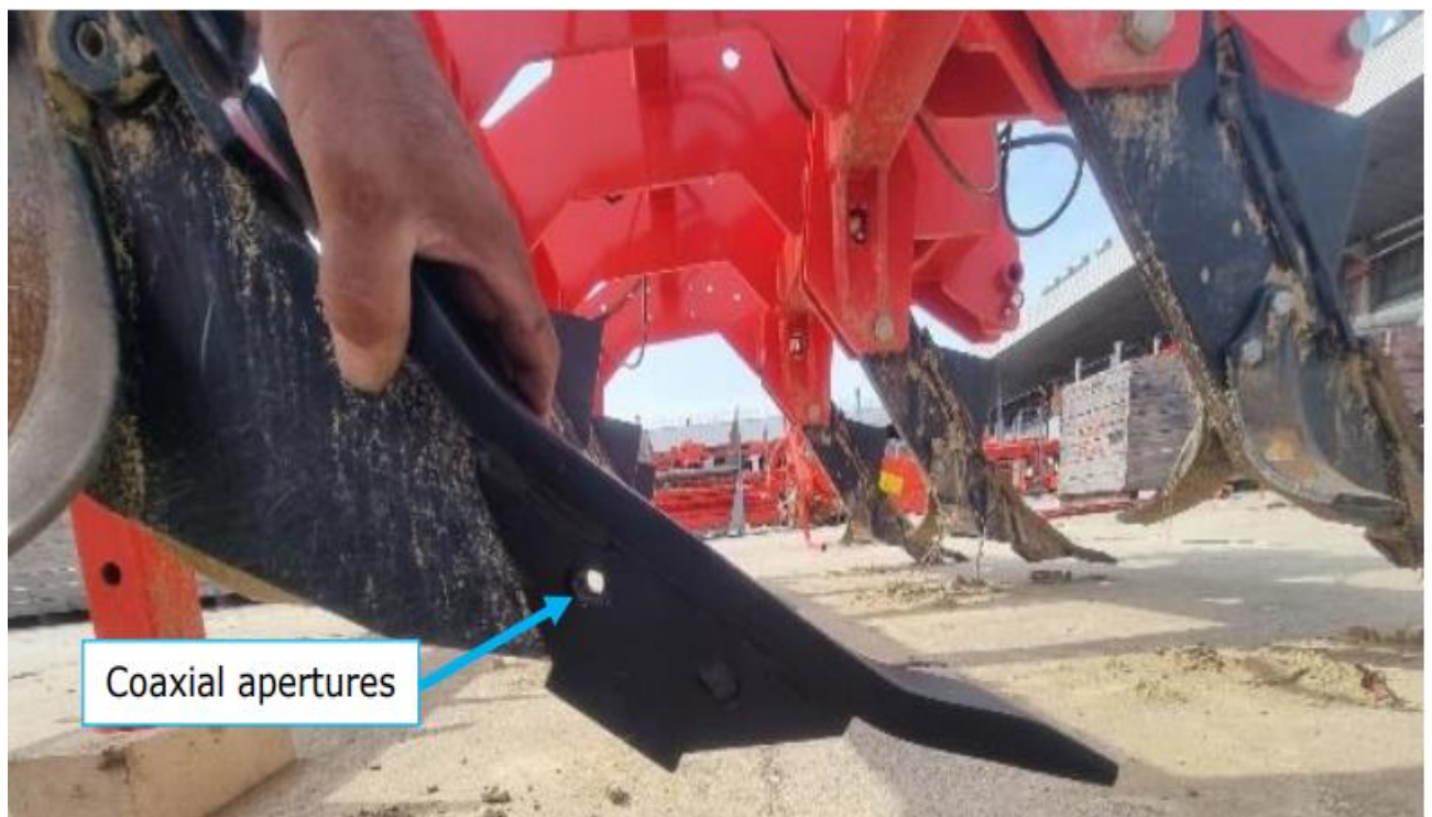
Figure 25. Lateral view of the Bellota tool mounted on the MG anchor member.
