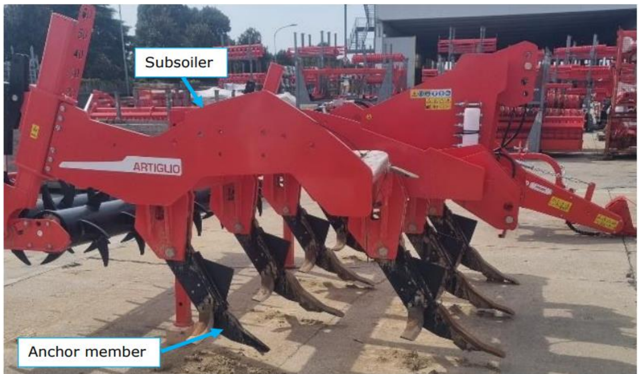
Figure 15. View of a MG subsoiler with anchor members onto which the Bellota tool can be mounted.
